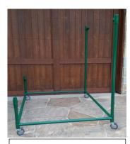
Step #3: Form the base with 2 straight pipes in front and back. Insert the 4 vertical pipes.
