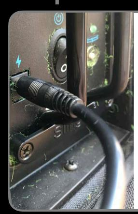
Plug power charger into the charger connector.
