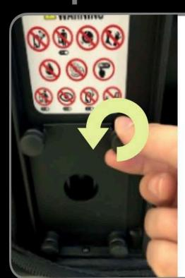
Place battery drawer back into the battery housing structure. Screw in the four battery drawer screws and tighten by hand.
