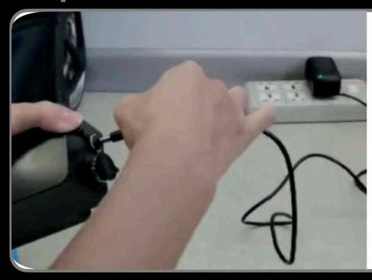
Plug power charger into the charger connector.
