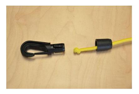
**4)** When repaired, the bungee and bungee clip will snap seamlessly together and will look like the photo below. Pull apart with moderate force to test.
